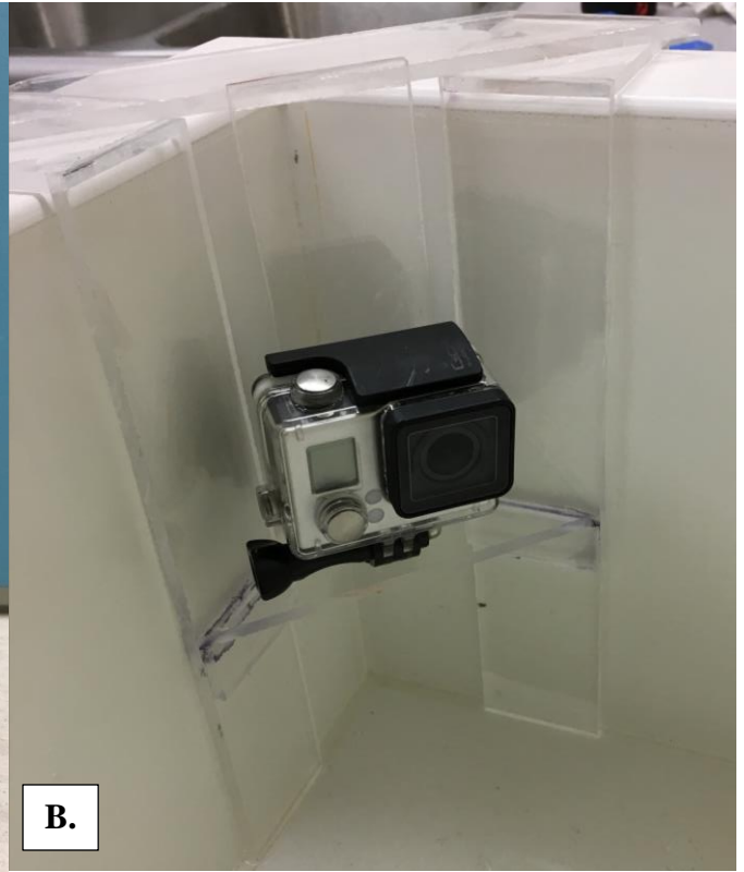
Figure 3. Example of plexiglass frames (A.) that secured cameras (B.) to the corners of observation tank.
